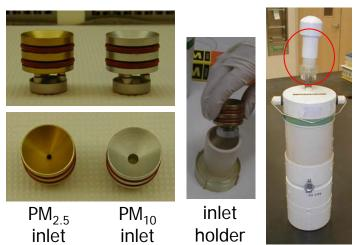
Figure 3.3: Minivol sampler and PM filter assembly
