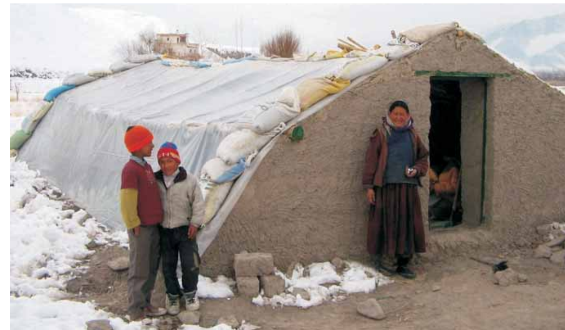
Passive Solar Greenhouse in a Land Covered by Snow in Basgo
