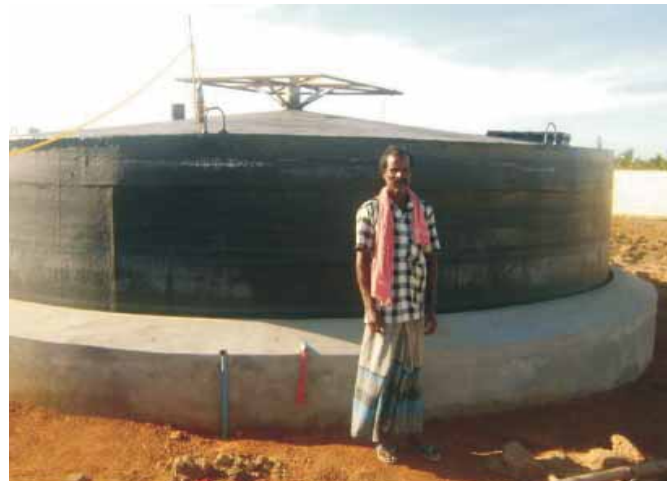
100 cm 3 Biogas Plant with FRP Gas Holder
