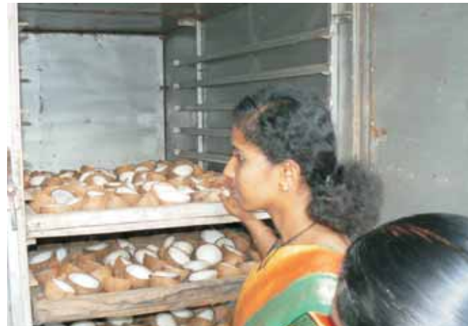
Biomass Dryer for Drying Coconuts
