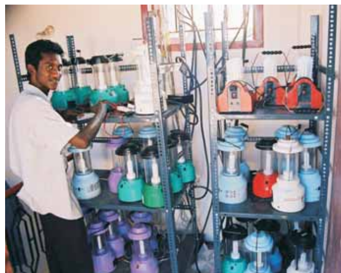
Recharging unit of Solar Lanterns
