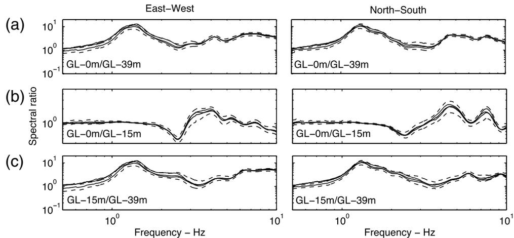
**Figure 4.** Average spectral ratio of (a) GL-0m/GL-39m, (b) GL-0m/GL-15m, and (c) GL-15m/GL-39m for north-south (right) and east-west (left) components for the frequencies with a Signal-to-Noise ratio over 3. The black continuous line shows the average ratio (+/- standard deviation in dotted line) for the time window including  $P$  and  $S$  waves. Superimposed gray lines show the average ratio for time windows including only  $S$  waves or Coda waves.
