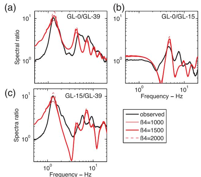
**Figure 5.** Comparison between the observed north-south spectral ratio (black) and computed (red) at the vertical array (Belleplaine test site) using the Kennett (1974) method: (a) GL-0m/GL-39m, (b) GL-0m/GL-15m, (c) GL-15m/GL-39m, using three values of  $S$ -wave velocities in the bedrock layer.
