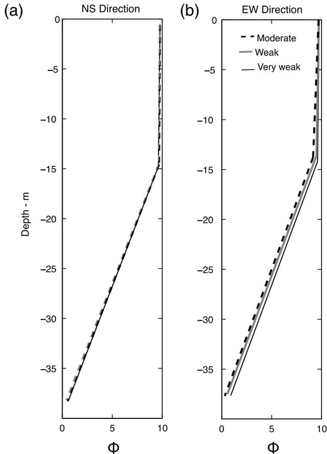
**Figure 6.** Experimental first mode in the (a) north-south and (b) east-west directions, using the FDD method and for three ranges of peak ground acceleration (moderate:  $\text{PGA} > 0.35 \text{ cm/s}^2$ ; weak:  $0.15 < \text{PGA} < 0.35 \text{ cm/s}^2$ ; very weak:  $\text{PGA} < 0.15 \text{ cm/s}^2$ ).
