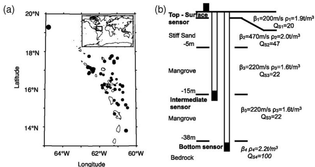
**Figure 1.** (a) Epicenters of the earthquakes recorded at the Belleplaine test site and used in this study. (b) Description of the soil profile and position of the accelerometric sensors.
