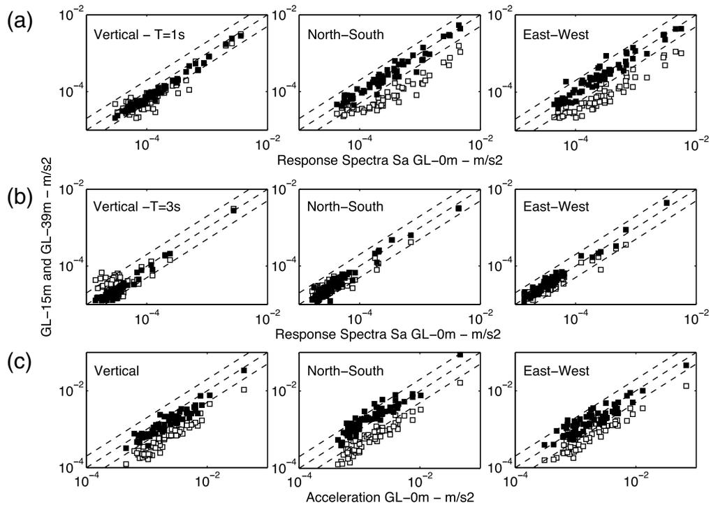
**Figure 3.** Seismic ground motion recorded at GL-39m (open squares) and at GL-15m (filled squares) as a function of surface ground motion (GL-0m) for vertical (left), north–south (middle), and east–west (right) components. (a) Accelerometric response spectra at 1 s. (b) Accelerometric response spectra at 3 s. (c) Peak ground acceleration (PGA).
