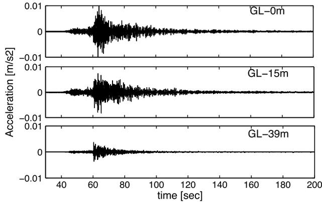
**Figure 2.** Example of north–south recordings at the three GL sensors ( $M_L = 6.4$  at 80 km).
