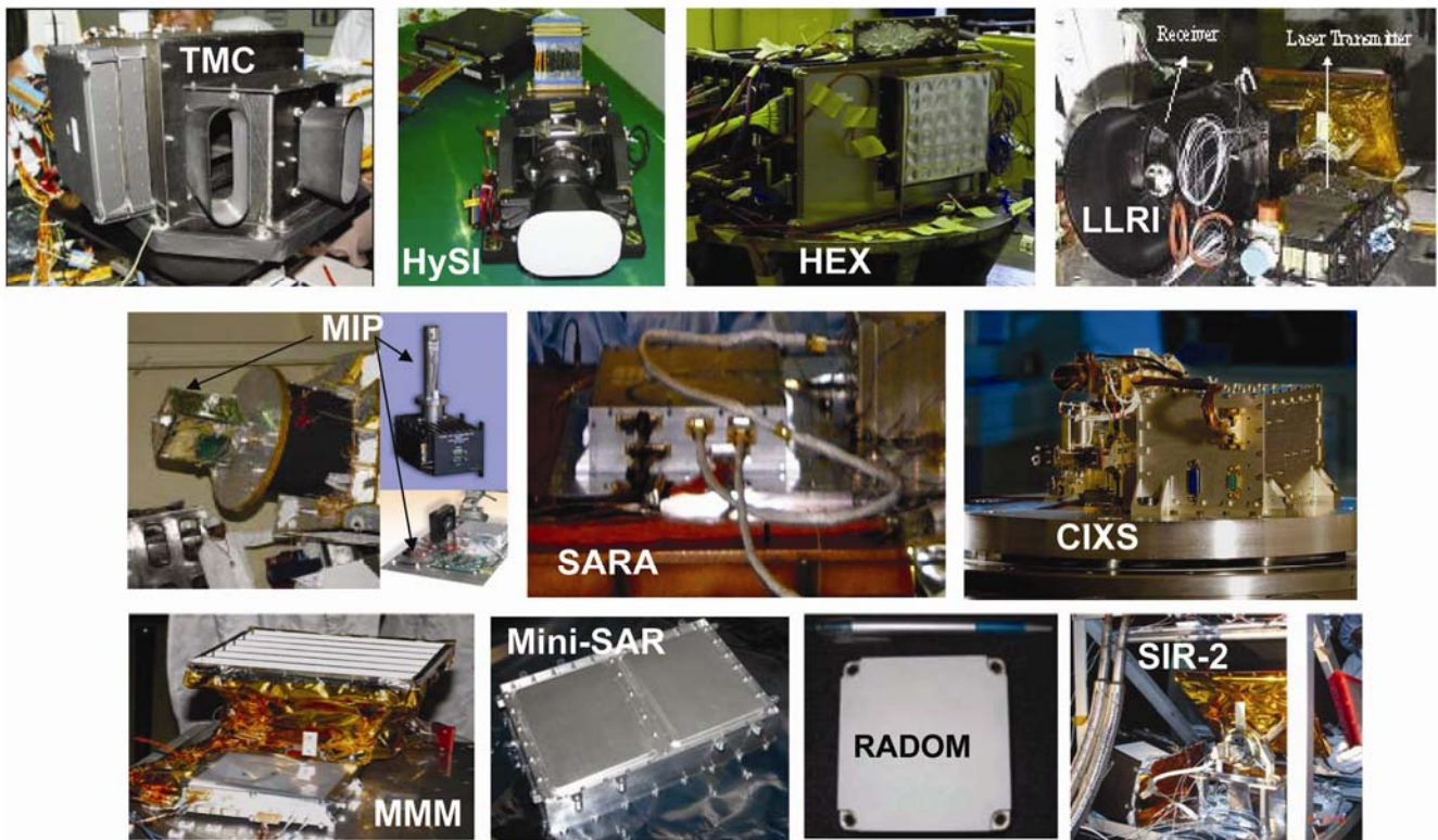
Figure 3. Flight model of the eleven payloads on board Chandrayaan-1. Four of the Indian payloads (TMC, HySI, HEX and LLRI) are displayed on the top panel; the middle panel displays the Moon Impact Probe and two of the instruments on it along with two AO payloads (CIXS and SARA from ESA) that have significant Indian collaborations. The four payloads shown in the lower panel are AO payloads provided by NASA (Mini-SAR, MMM), ESA (SIR-2) and BSA (RADOM).
