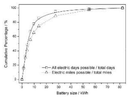
Figure 14 : Proportion of trips possible from batteries of different capacities
