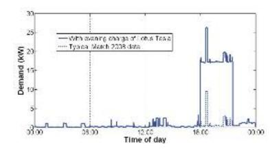
Figure 25 : Power demand (with EV) - scaled to 30kW
