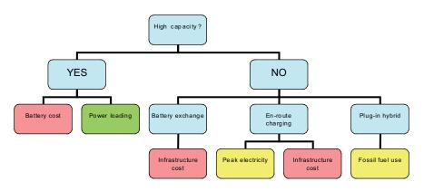
Figure 26 : Choice of battery capacity
