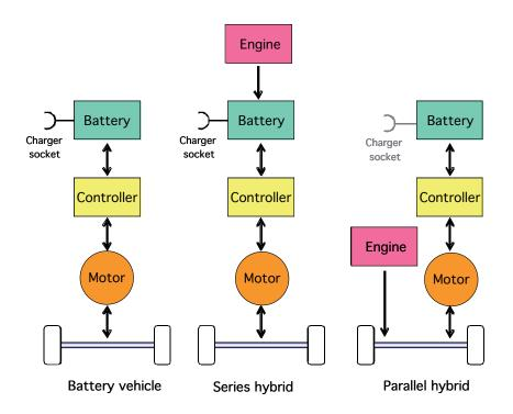
Figure 17 : Alternative hybrid configurations
