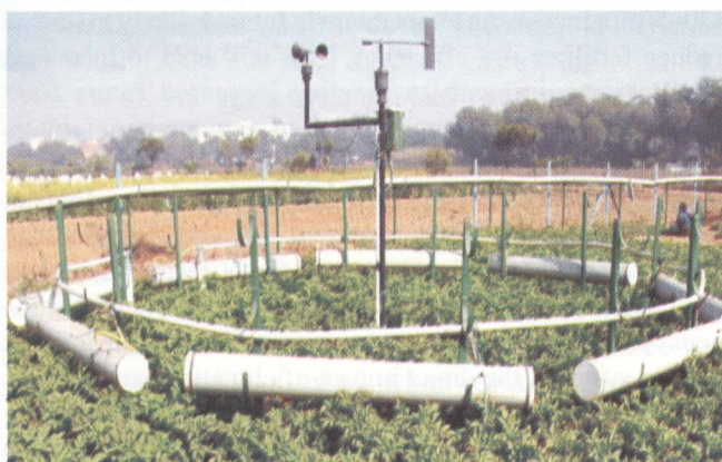
Fig 3 Free-Air - Carbon dioxide-Enrichment (FACE) setup at the Indian Agricultural Research Institute to study the impact of increased CO 2 on crops
