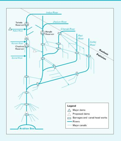
network is massive, with 43,561 kilometres of canals, 18,884 kilometres of seepage/storm water drains and 12.612 kilometres of tile drains, mostly in the Indus Plain provinces of Punjab and Sindh. This system of reservoirs and canals forms the basis of the Indus Basin irrigation system and is thus absolutely essential to agriculture.
