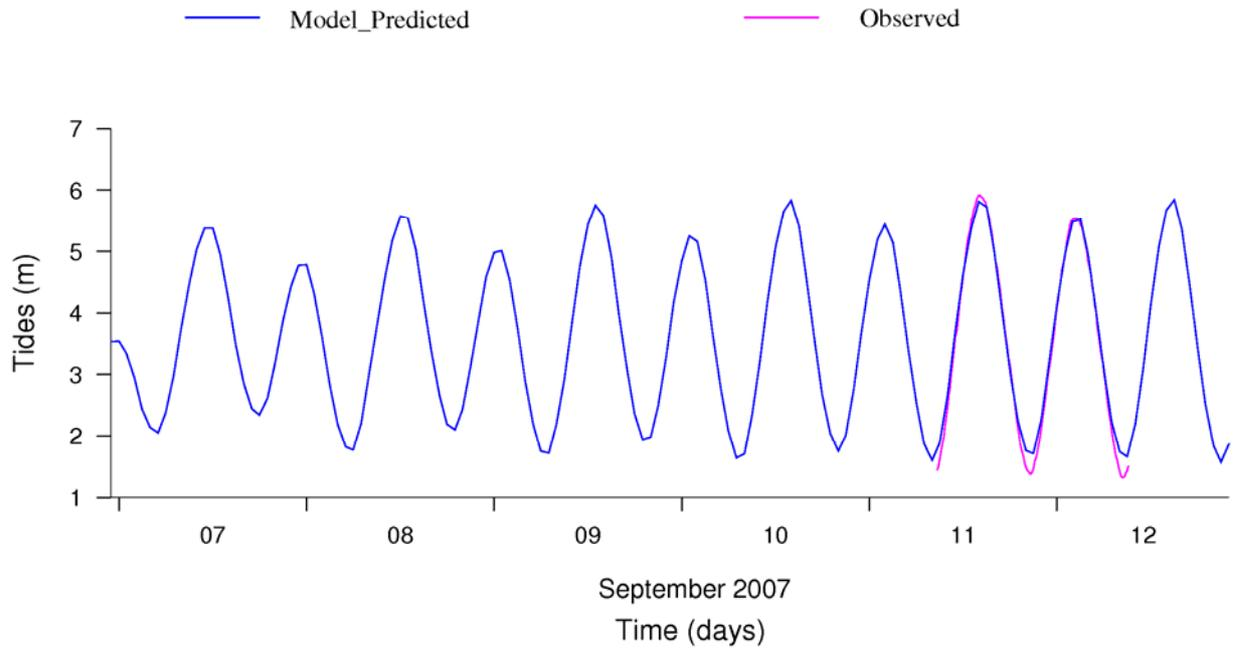
Fig.6 Comparison of computed and measured tides at Bhadreswar
