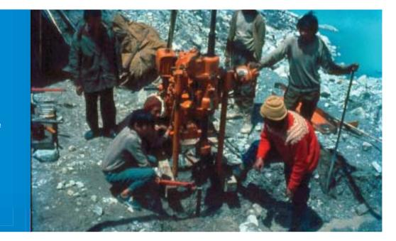
**Fig.9:** Deep drilling for ice core recovery in progress on a glacier in the Himalayas.
