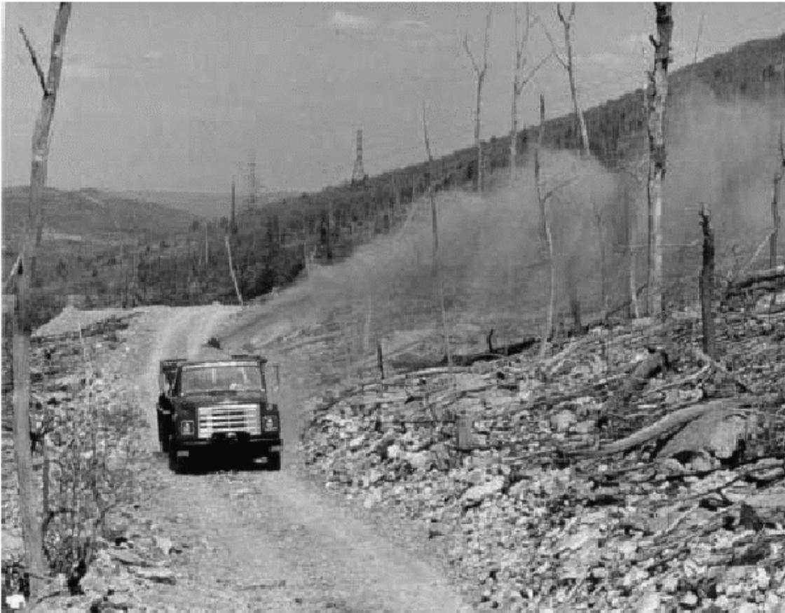
Spreader fan distributing a mixture of biosolids and fly ash on the Palmerton, PA Site
