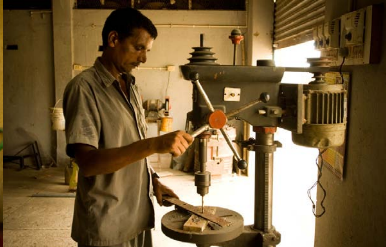
Image: Fitter Damodar Sharma operates a drilling machine in the research lab of Solar Alternatives and Associated Programmes. All machines in the workshop run on electricity generated through solar photovoltaic panels on the workshop roof.
