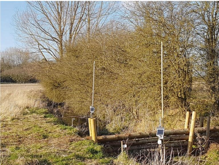
**Fig. 4.1** Live FreeStations monitoring water level and soil moisture upstream and downstream of a Leaky Dam (*left*) and close-up of a water level FreeStation (*right*). Each has a pole-mounted aerial to improve mobile connectivity
