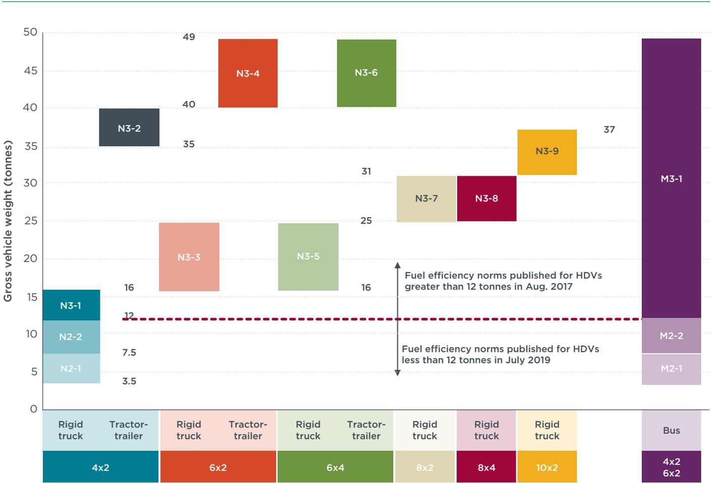
Figure 10. Categorization scheme in India's fuel efficiency regulations for commercial vehicles
