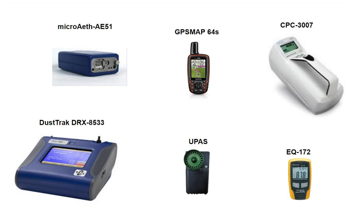
Figure 1: A collage of instruments used for on-road air pollution monitoring (source: tsi.com, garmin.com; aethlabs.com; accsens.com)
