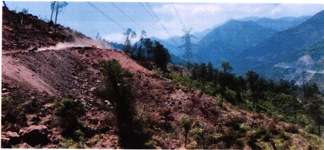
Fig. 7. Illustrating landslide affected slope; the displaced debris composed of clasts of mudstone, siltstone, and boulders of sandstone.
