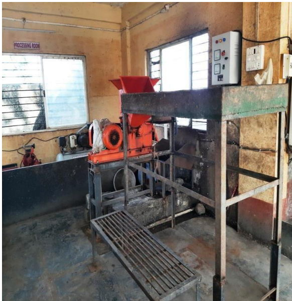
Photograph-3: Shredder for handling solid waste (Type-I & II) prior feeding to the biogas plant.
