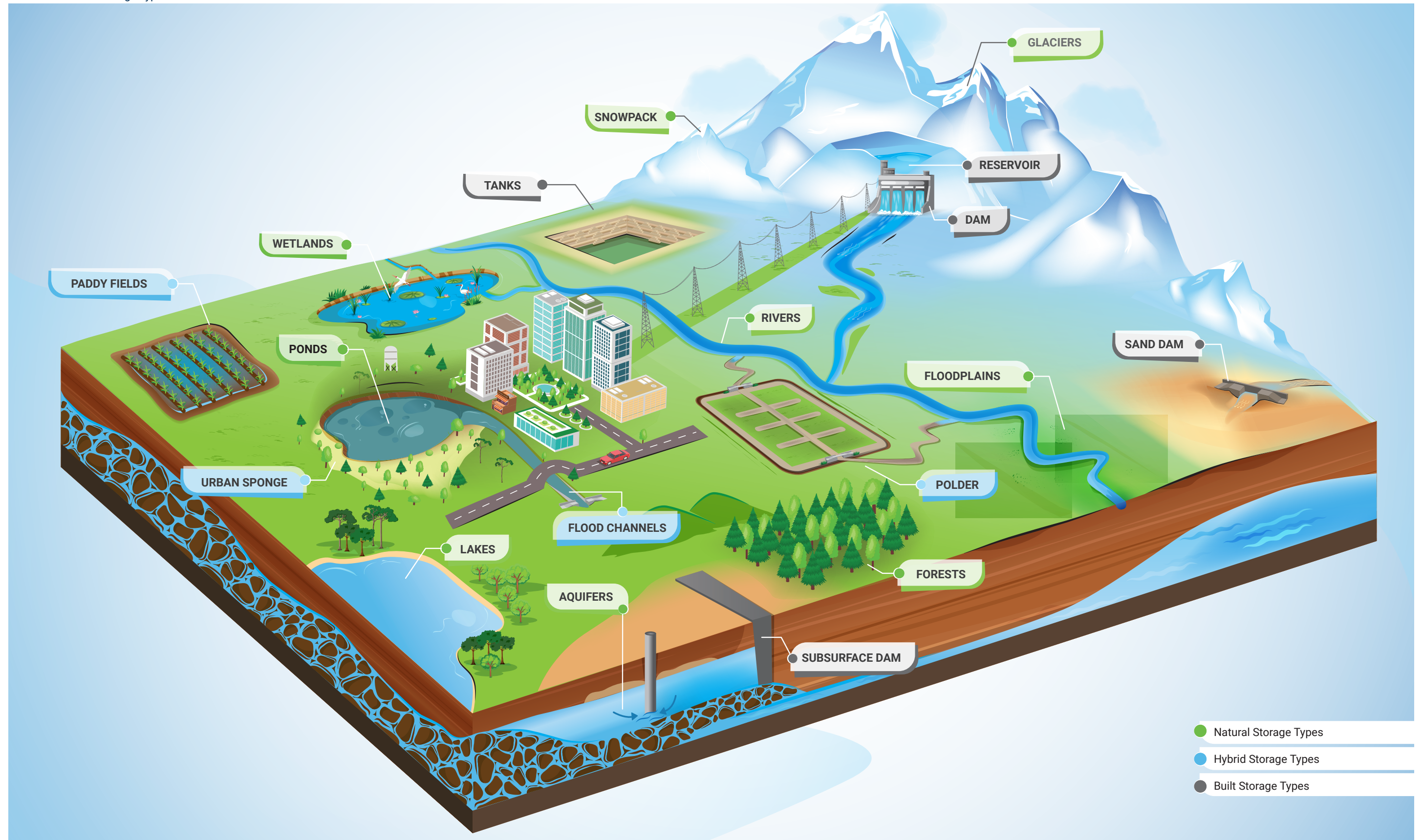
FIGURE 2.1 Water Storage Types
