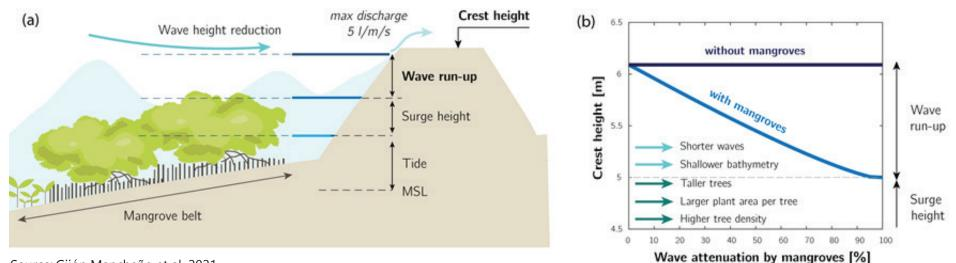
Figure 6.37: Design Water Levels (left) and Required Embankment Height (right) with and without Wave Attenuation by a Mangrove Belt (Polder 56/57)
