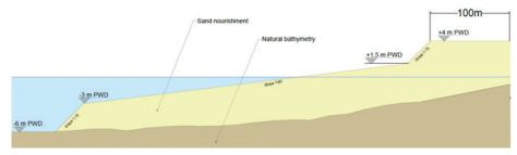
**Figure 6.25:** Intervention Layout of Kolatoli Beach with Sand Nourishment and Multifunctional Embankment
