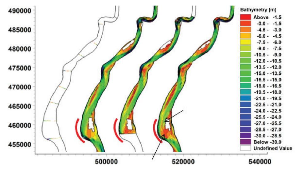
Figure 6.7: Observed Bed Topography of the Baleshwar River during (from left to right): 2009, 2011, 2015, and 2019
