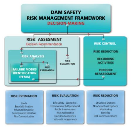
Note: Potential failure modes analysis (PFMA)" Source: US FEMA 2015.
