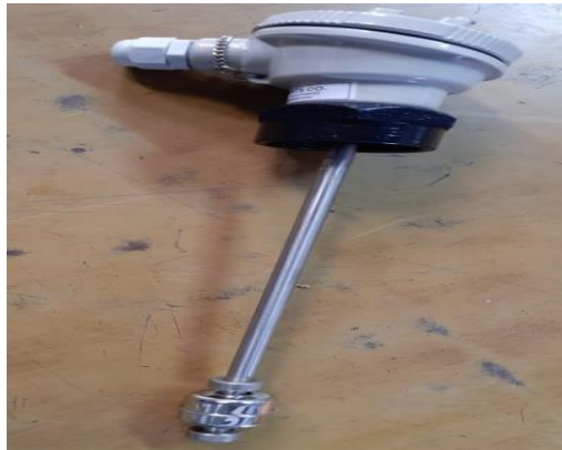
Fig. 2: Float sensor for oil-level monitoring.
