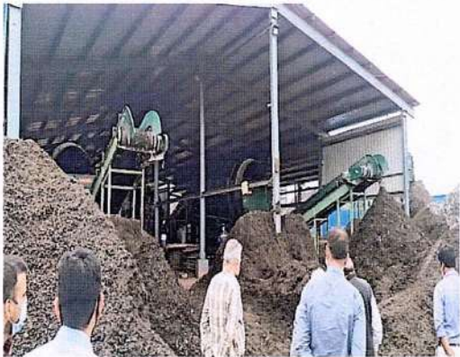
Plate-2: Photograph showing the machinery in operation for processing of legacy waste
