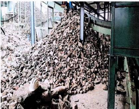
Plate-3: Photograph showing RDF produced by processing of legacy waste
