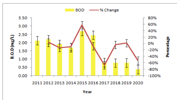
Fig.. 3.12: Yearly Average Concentration of BOD and rate of Change in BOD in different districts of H.P from 2011-2020 ( Source-Himachal Pradesh State Pollution Control Board (HPSPCB) )
