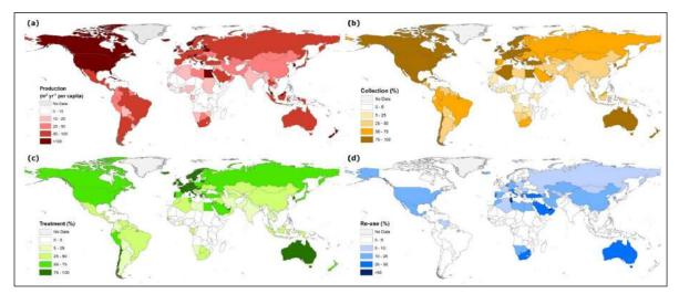
Figure 2.1.3: Global wastewater estimates at country scale: a) Wastewater production (m3/year per capita), b) wastewater collection (%), c) wastewater treatment (%), and d) wastewater reuse (%) (Source: Jones et al., 2020)
