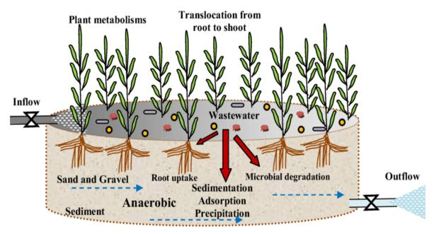
Figure 4.2.2: Pollution removal mechanism for constructed wetlands
