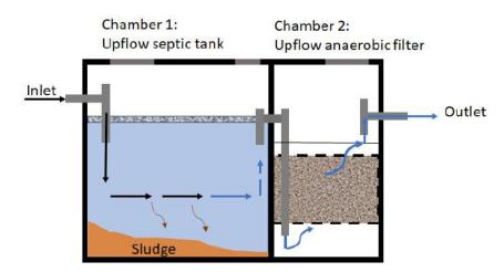
Figure 4.3.5: Modified septic tank-anaerobic filter unit as a two-stage on-site domestic wastewater treatment system
