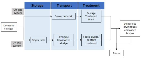
Figure 3.3.1 : Storage, transport, and treatment mechanism of an off-site and on-site wastewater treatment system
