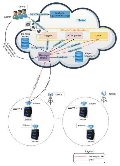
Figure 4.3.1: EcoSens Aquamonitrix Smart Wastewater Quality Monitoring System (Source: Martínez et al., 2020)
