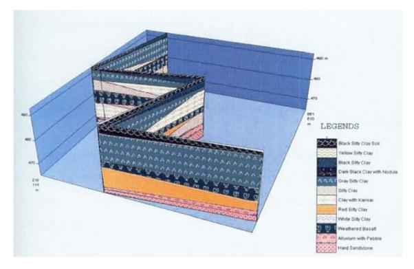
Figure 12: Fence diagram showing geological strata at UCIL premises
