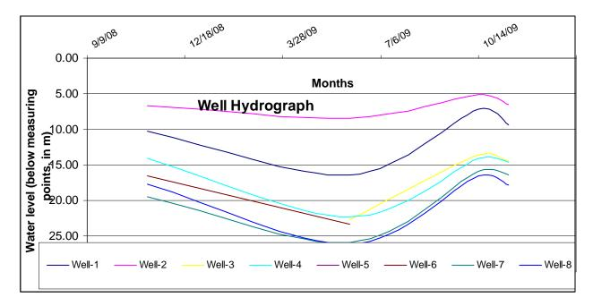
Fig. 7 Well Hydrograph of wells at the periphery of area
