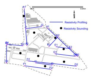
Fig. 4: Resistivity profiling & soundings during 1994
