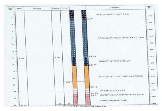
Figure 10: Litholog and drill-time log at bore well D
