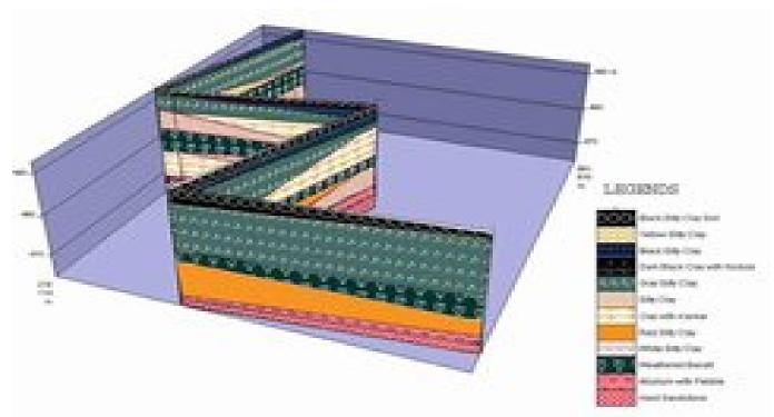
Fig 14 Fence diagram showing geological strata
