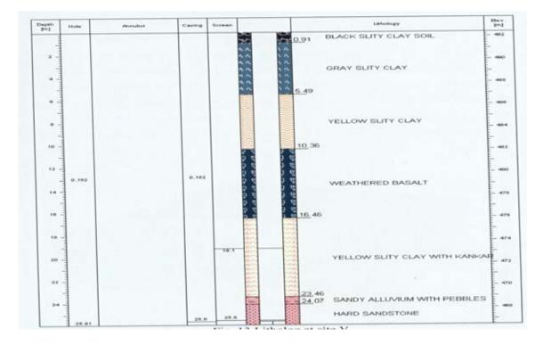
Figure 11: Litholog and drill-time log at bore well E
