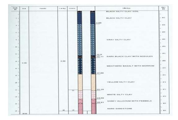
Figure 7: Litholog and drill-time log at bore well A
