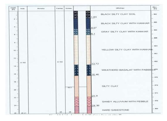
Figure 8: Litholog and drill-time log at bore well B
