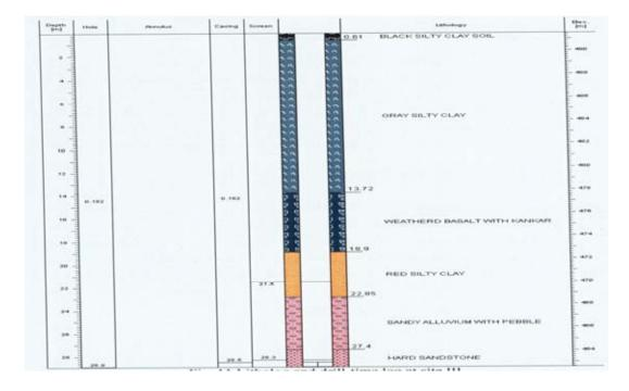
Figure 9: Litholog and drill-time log at bore well C
