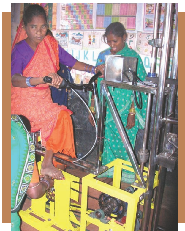
Pedal-powered biodiesel processor
