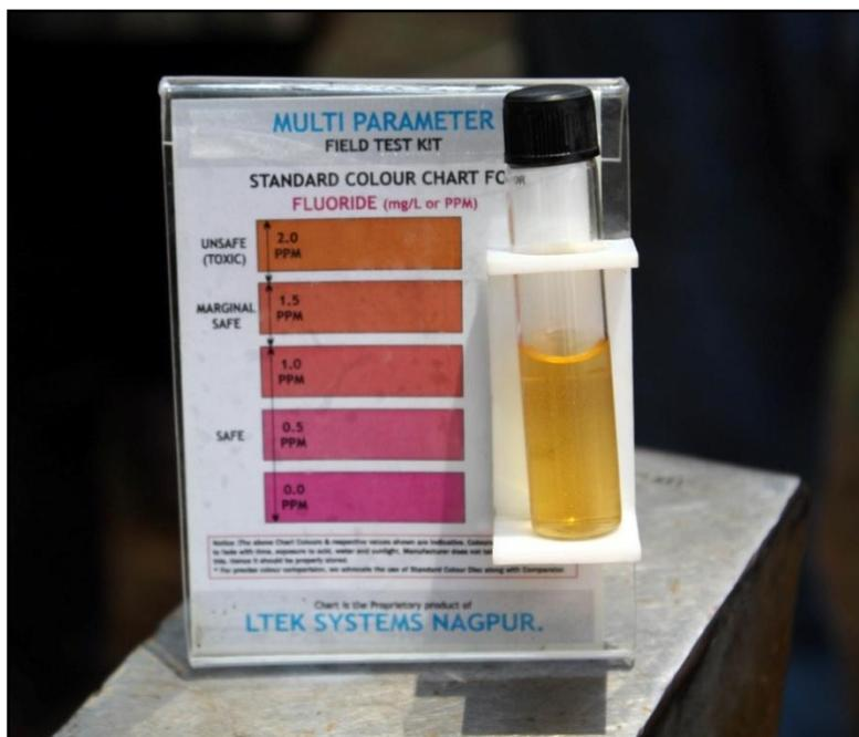
**Photo 9:** A water sample from a handpump showing a high fluoride content.
