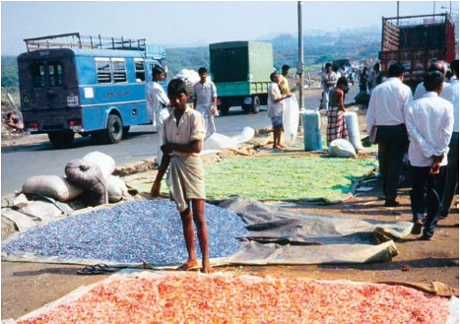
Photograph 3: This recovered plastic has been sorted by type and colour, cut into small pieces and washed, and it is now drying in the sun, in preparation for further processing
