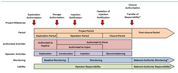
Figure 2: The life cycle of a CCS project as adopted by this *Model Framework*
