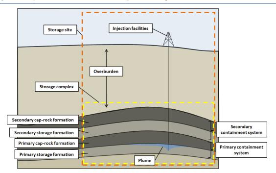
Figure 3: Components of the sub-surface that may be used in legal definitions
