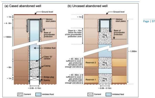
Figure 8: Example of how cased and uncased wells are abandoned today
