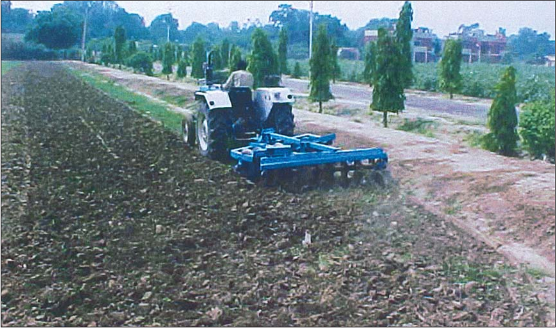
Figure 4. Land preparation with tractor drawn disc plough useful in reducing time between harvesting and planting in CWPS.
