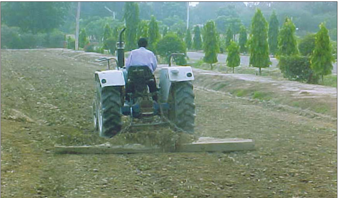
Figure 5. Tractor drawn planking operation as a part of quick land preparation.
