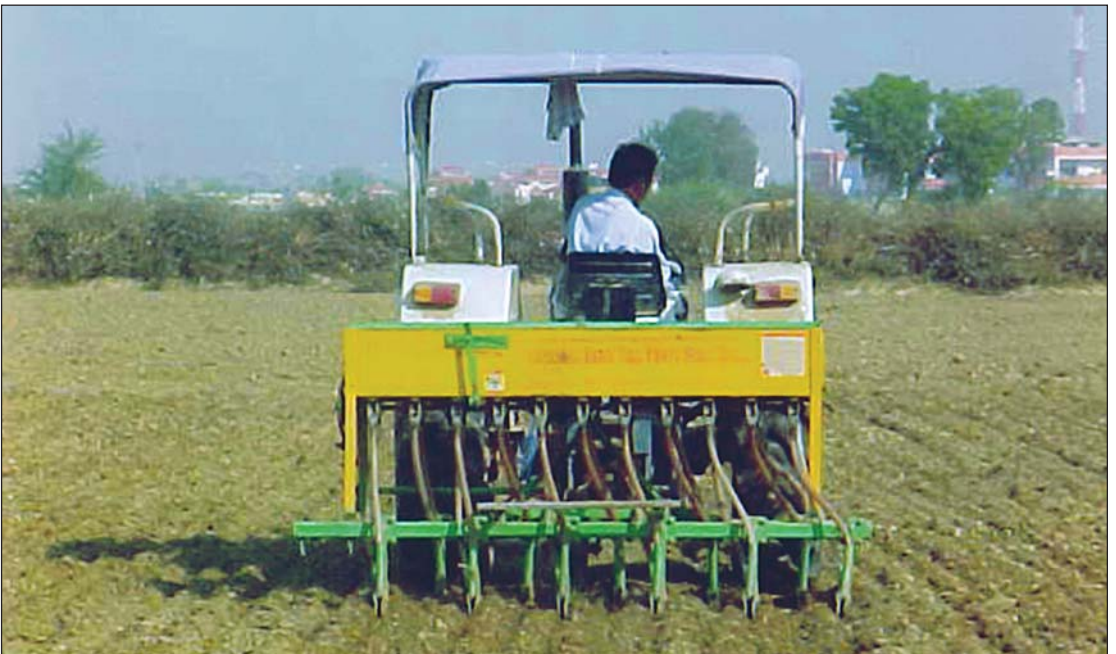
Figure 7. Zero-till planting of wheat: a resource conservation technology extremely useful in CWPS.
