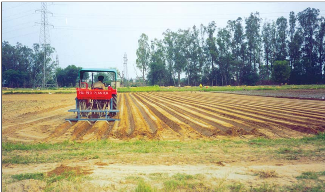
Figure 8. Mechanical bed preparation for simultaneous operations of tillage and sowing useful in cotton and wheat cultivation.
