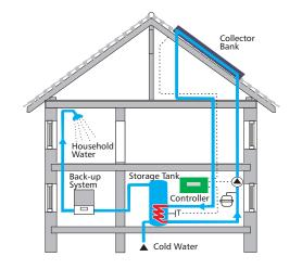
Fig4: Forced circulation with heat excghanger
