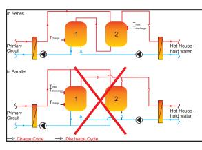
Fig12: Interconnection of storage tanks
