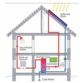
Fig5: Forced circulation with heat exchanger
