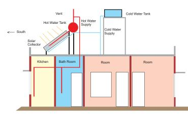
Fig2: Thermo siphon system with over head tank
