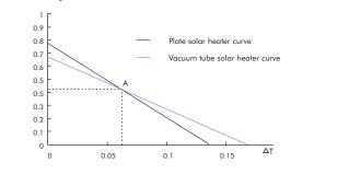
In the figure, the Y axis represents efficiency of the solar collector and X axis represents ratio of temperature difference to the solar radiation. Therefore,  $\Delta T = (Ti-Ta) / G$
