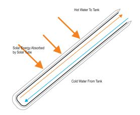
Fig20: Double Glass Evacuated Tube with inner tube coated and filled with water.
