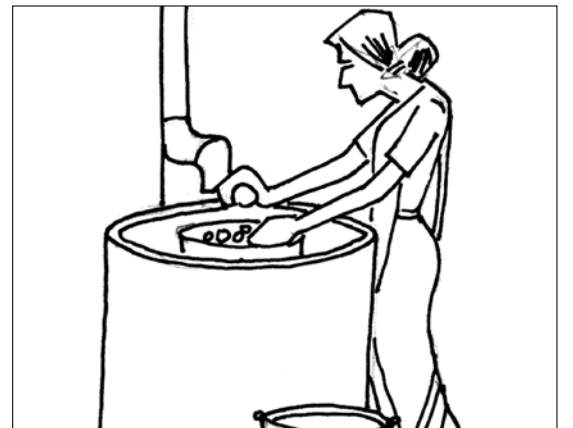
The filter tank needs to be kept clean
