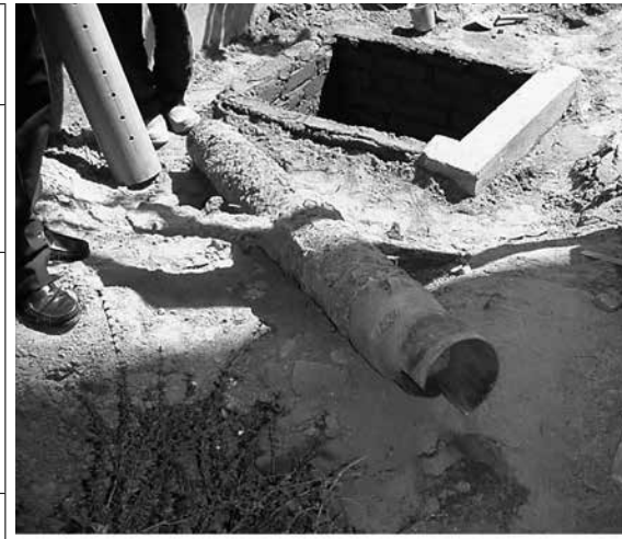
Casing of tubewell (top), slotted pipe (below)
